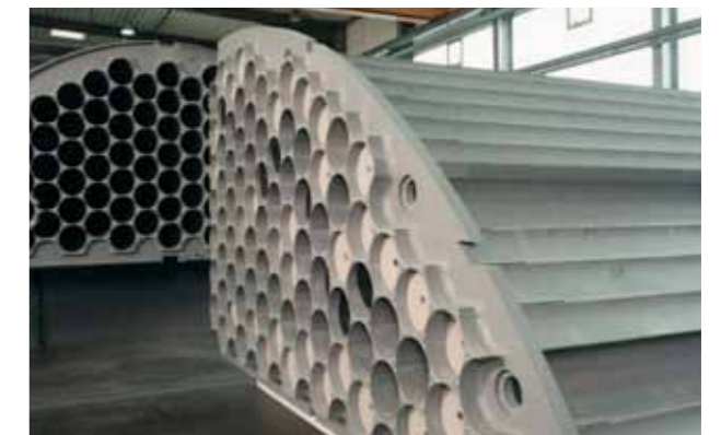
Oben: Patented tube bundle for wet electrostatic filter.
