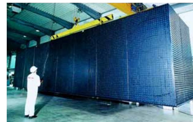
Above picture: Pre-fabricated BEKAPLAST™ tank made of HDPE for concreting into place on site.
