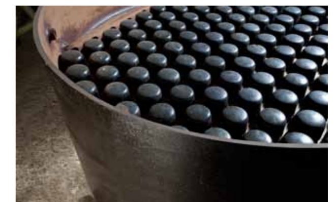
Above picture: KERA Column strake with built-in bubble tray.
