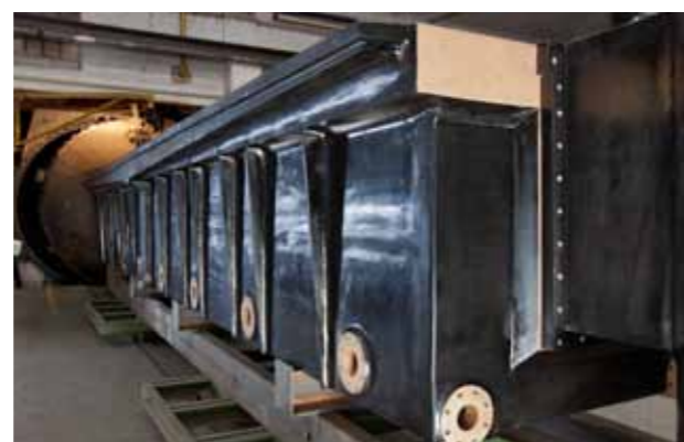
Above picture: Vat made using solid KERA for spun fibre industry.
