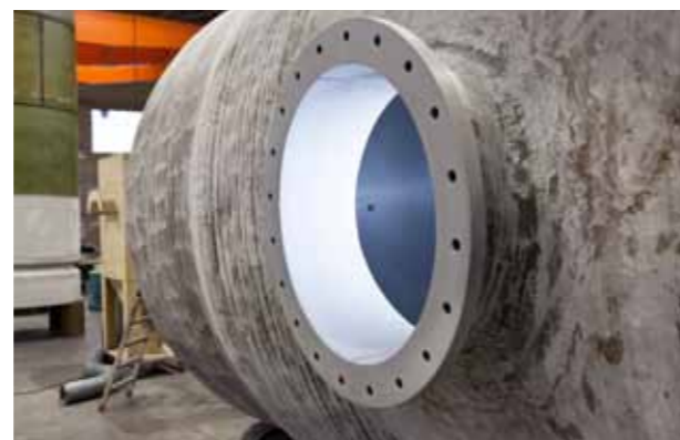
Above picture: Process tank made of PTFE and glass-fibre reinforced plastic.
