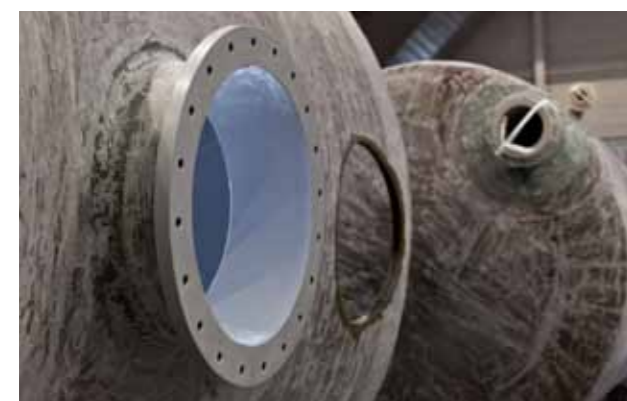
Above picture: Tank made of PVDF and glass-fibre reinforced plastic in manufacturing process.
